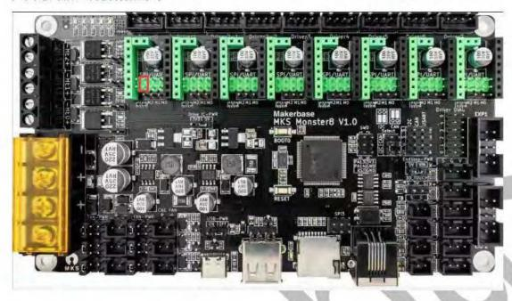
Note: Based on Voron V2.4, in order to facilitate the drive current adjustment, the default configuration of the mks monter8 V1.0 motherboard (the configuration obtained on the mks qq group or mks github) is to enable 7 TMC2209 UART modes, so use it directly The default configuration requires 7 drivers to be set to uart mode.
