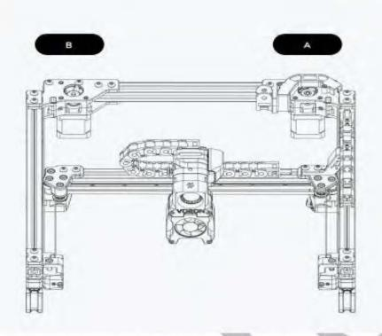
Note: Please be sure to follow the above wiring. Wrong wiring of A and B motors will cause movement errors, printing mirror images, etc., wrong 4Z sequence connection will cause incorrect leveling.
