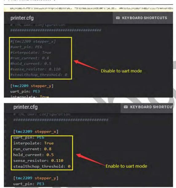
Note: The configuration enable is uart mode, which requires hardware support, uart mode drives jumpers, see 2.4 for details
